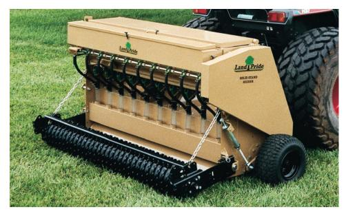
When the optional small seeds box is used, two seeds can be metered at one time. The two seeds are metered into the same seed tube for even distribution.
